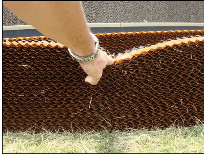
Figure 5. Pad constructed of poor quality paper.
